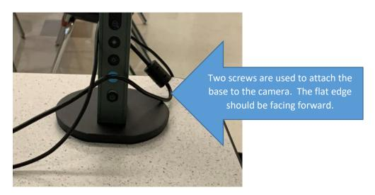
2. Plug the cord into the back of the document camera and into the USB port on the side of your Surface.
