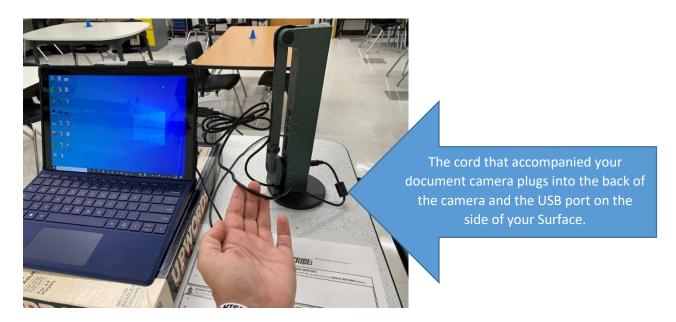
3) Open the camera arm and position it as desired. You can also flip the camera head itself up and use it as a "web cam" to record yourself (3). The camera head can also swivel (4).
